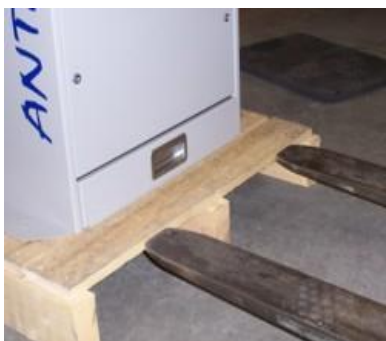
3. Position Fork Lift extensions in-line with pallet top.
