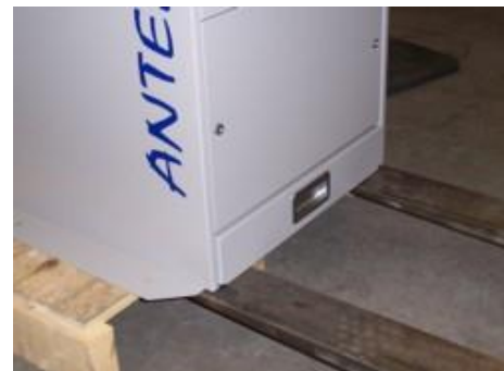
4. Slide the machine onto the fork lift extensions.
